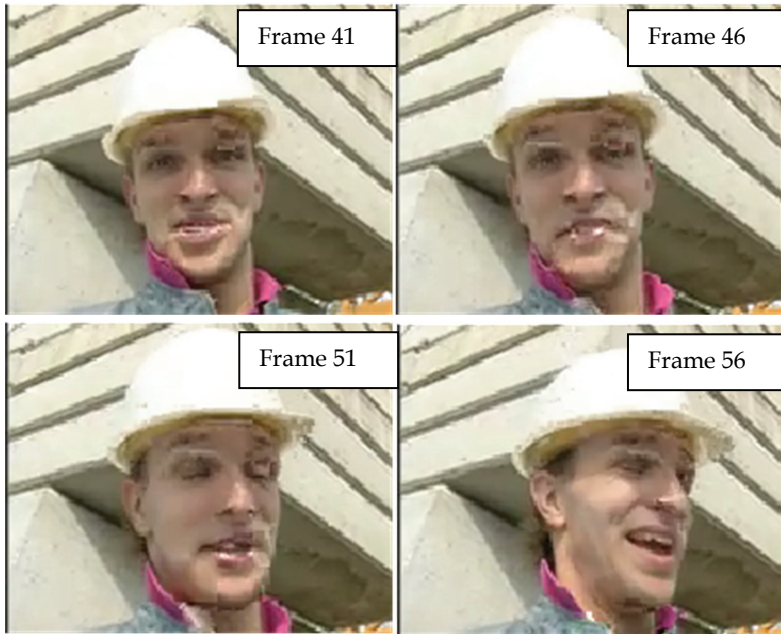
Fig. 2. Error propagation in standard H.264/AVC caused by a single bit error
