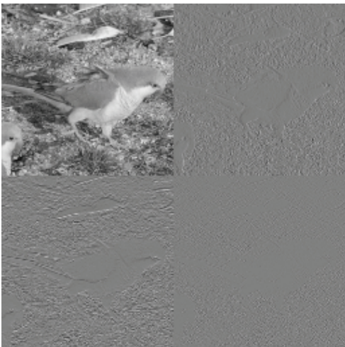
Fig. 1.9. Columns wavelet decomposition
